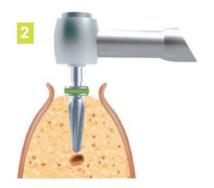
Drill at 150 rpm without **irrigation** or at 650 rpm **with irrigation**. Use the drill Ø 3,6 mm.
