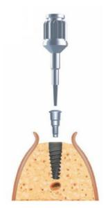
Screw the cover screw at 5 N.cm with the screwdriver P/N 0014 or P/N 0114.
